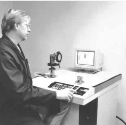
A lab service technician performs a helium leak test to verify fitting integrity.
