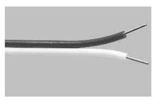
The SERIES 505 is the most economical wire produced. Unlike some competitive "ripcord" type constructions which use only a stripe to establish polarity, SERIES 505 single conductors are fully color coded. The conductors are individually insulated with the proper colored PVC and fused into "ripcord" using a proprietary process.
