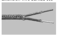
SERIES 305 is specifically constructed for light duty applications where size is a critical factor. The single conductors are insulated using a specialized yarn wrapped on the conductors in layers. This yarn is then impregnated to add abrasion resistance and enhance electrical properties. The insulated single conductors are then laid parallel and covered with a layer of braided glass. A final impregnation is applied to the braid.
